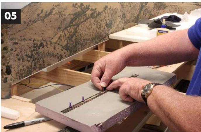
Image 05. Thumb tacks secure the track until the glue dries.
